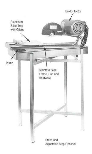
The journeyman tile saw has the most advanced drive system available—the pulley and cog belt is a high torque drive system. The bearings are double sealed for use in wet and dirty environments. The drive system is smooth running and delivers 20% more horsepower to the blade than conventional V-belt drives.
